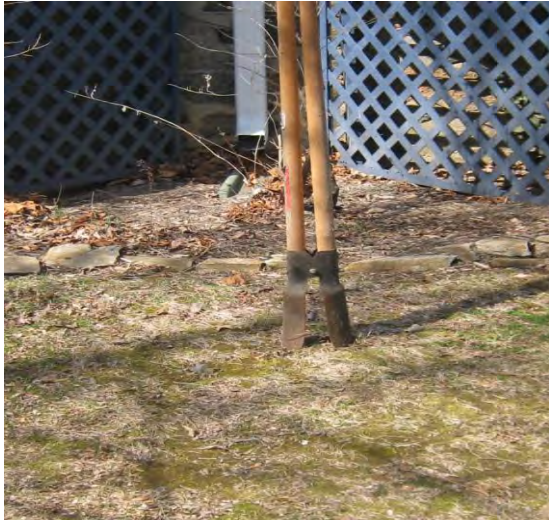
Post Hole Digger for Soil Test
