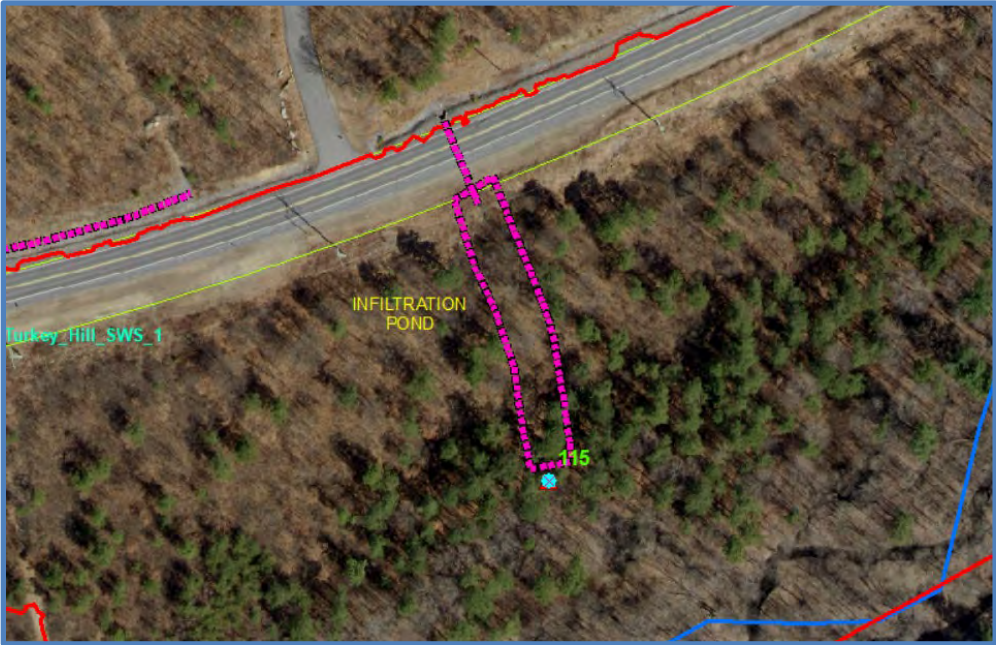
Outfalls 115 - 8 Turkey Hill SWS1: New BMP’s to address outfall from existing pipes.
