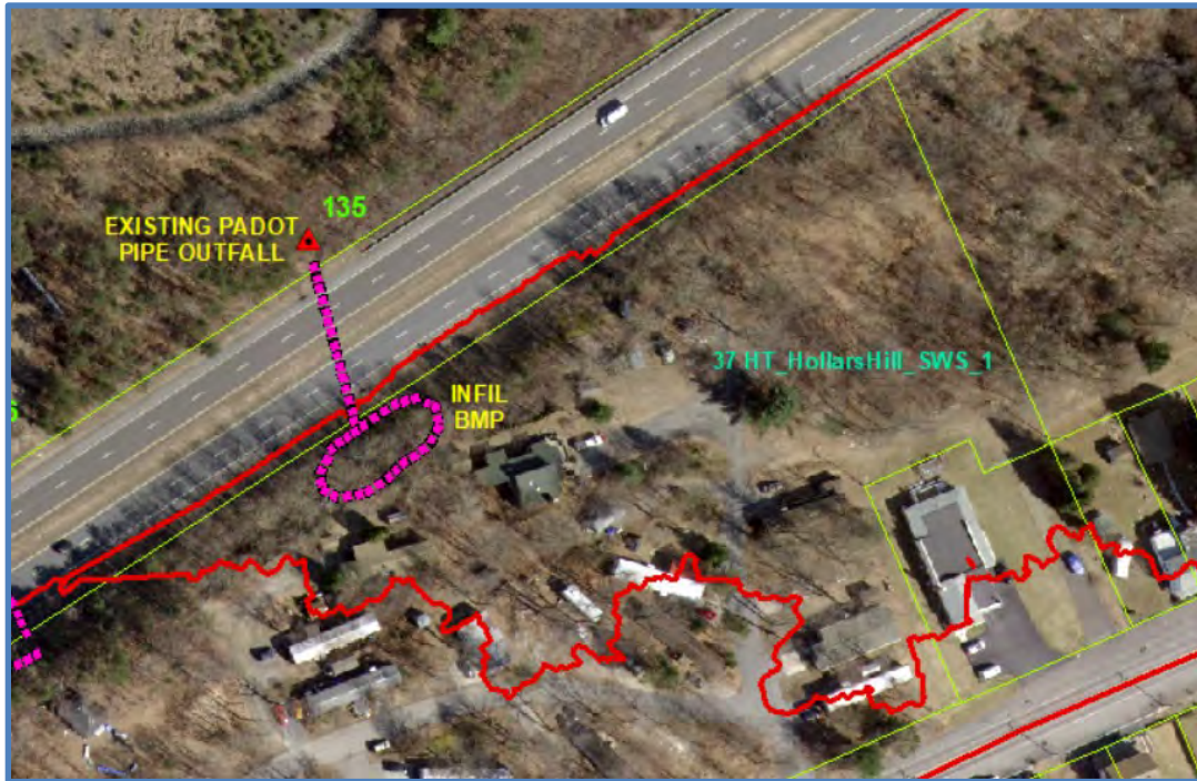
Outfall 135 - 37 HT Hollars Hill SWS 1: New BMP with Outfall to existing PaDot cross pipe.
