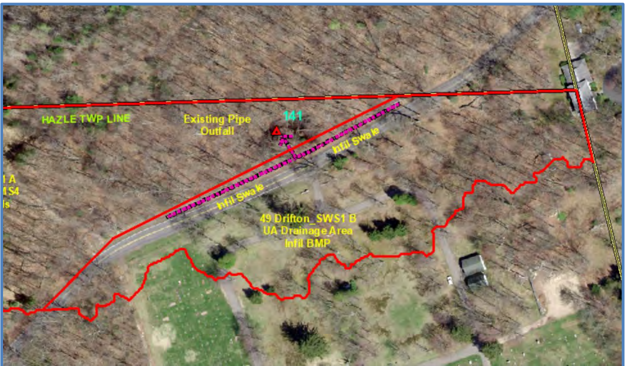
Outfall 141 - 49 Drifton SWS1: New BMP outfall from roadside swale.
