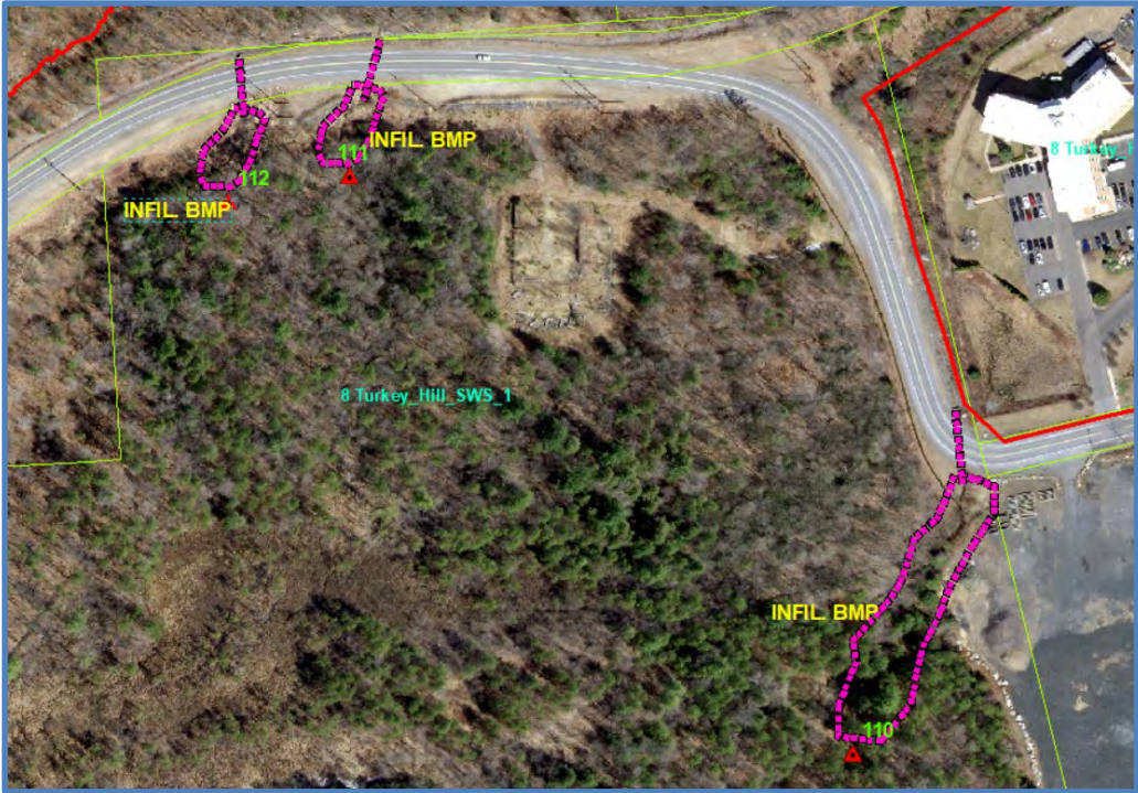
Outfalls 110,111 & 112 - 8 Turkey Hill SWS1: New BMP's to address outfall from existing pipes.
