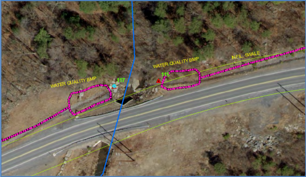
Outfalls 116 & 117 - 8 Turkey Hill SWS1: New BMP’s to address outfall from existing roadside swales at Black Creek.
