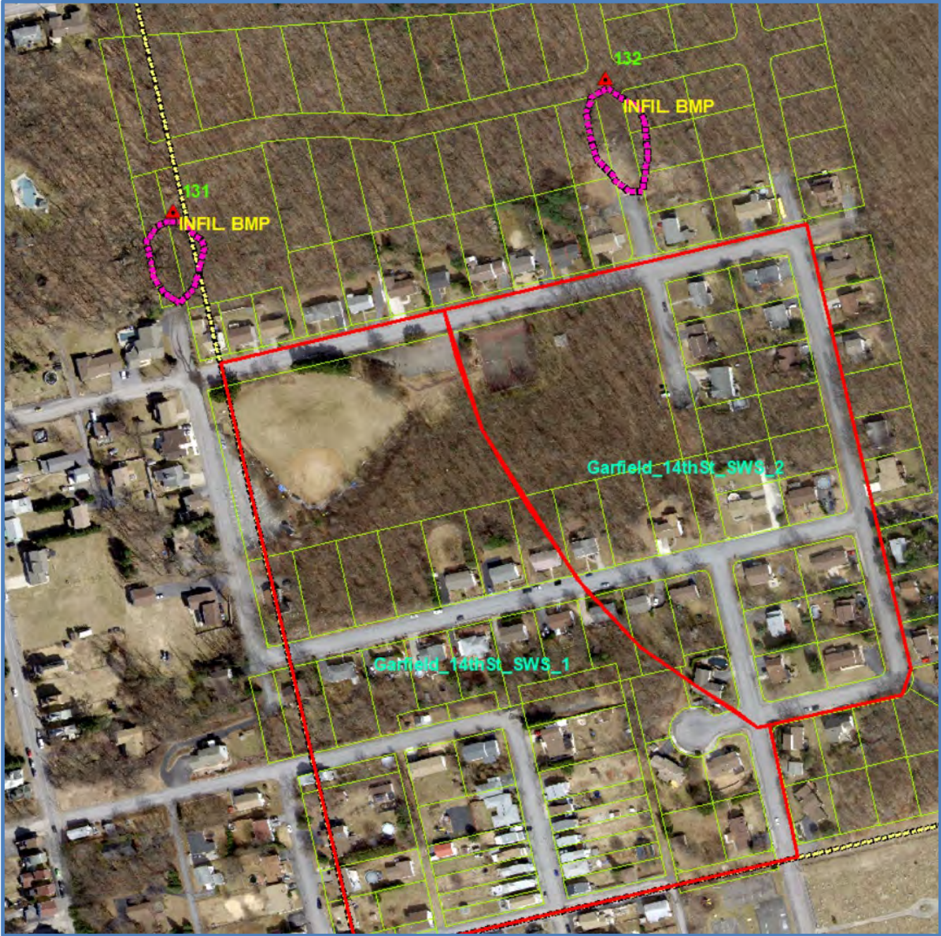
Outfalls 131 & 132 - 30 Garfield SWS 1 and 31 Garfield SWS2: New BMP outfalls to address stormwater runoff from existing pipes.
