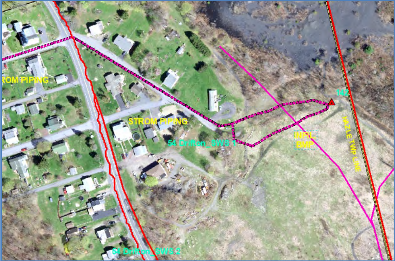
Outfall 142 - 54 Drifton SWS1 : New BMP outfall from roadside drainage system in Village of Drifton.
