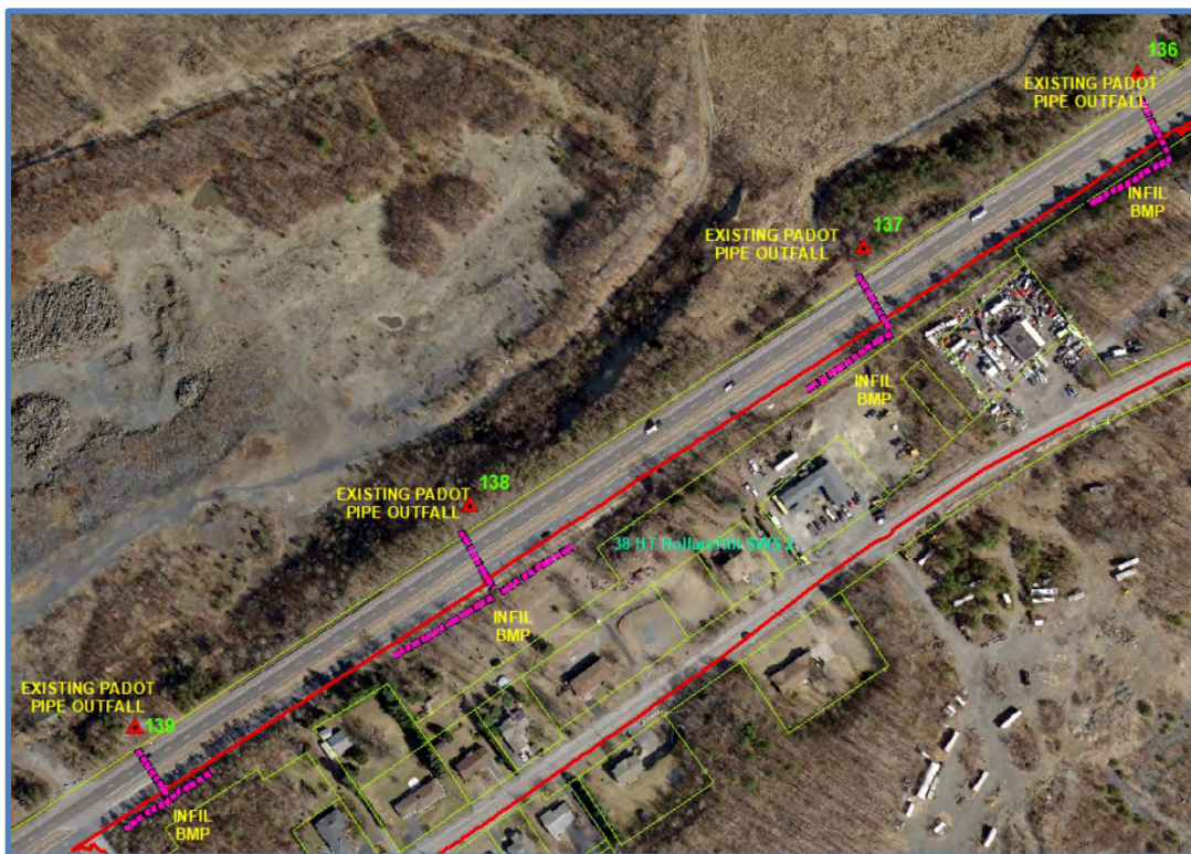
Outfalls 136, 137, 138 & 139 - 38 HT Hollars Hill SWS 2: New BMP's with Outfall to existing PaDot cross pipes.
