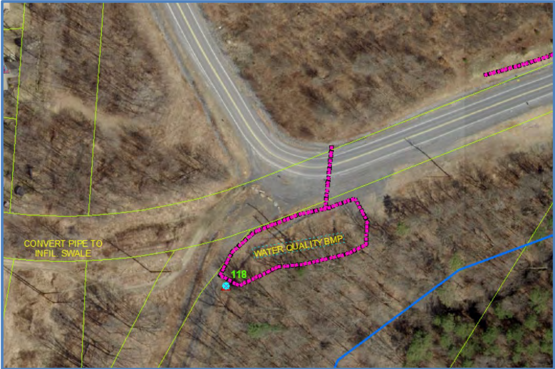
Outfalls 118 - 8 Turkey Hill SWS1: New BMP's to address outfall from existing roadside swales and cross pipe at Black Creek.
